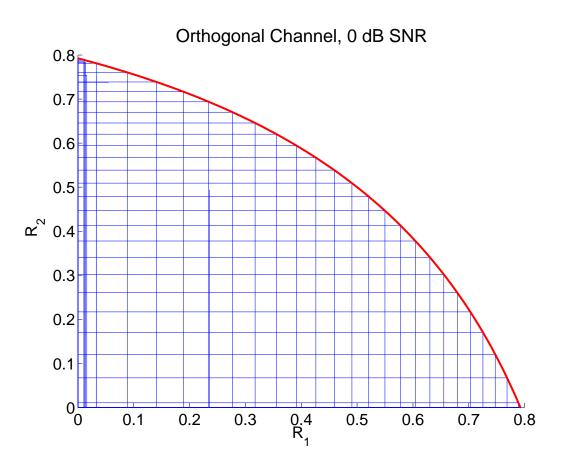
• in an orthogonal channel, TR works perfectly
